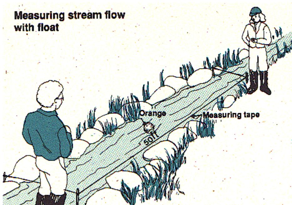
Measure off at least 50 feet along the bank of a straight section of stream. If possible, string a rope across each end of the 50-foot length.
